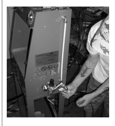
**Step 7**: Place magnetic hook on right and left side of the spray gun cleaner (leave the white cover on the magnets)
