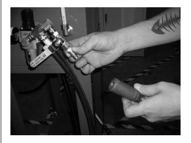
Step 9: Place a 5 Gal container (Used Solvent -Not supplied) on the shelf under the spray gun cleaner with black drain hose (for units with Optional Stand w/ Legs this hose will need to be trimmed by 10" – See Note) in center hole of the lid and suction line hose in the side hole of the lid. Note: Be sure the black suction line hose is all the way down to the spacer.
