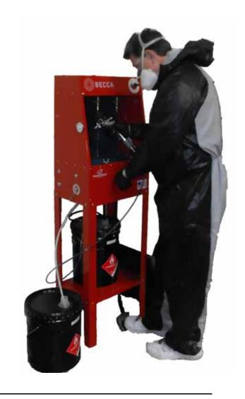
**Step 10**: Turn on ball valve to apply air to the system and adjust all air and fluid flow levels.
