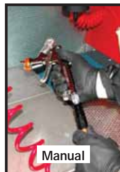
POWERCLEAN™ .... Supply's Compressed Air to the Spray Gun During the Cleaning Process, Protecting the Air Passageways
