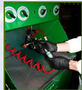
POWERCLEAN™ .... Supply's Compressed Air to the Spray Gun During the Cleaning Process, Protecting the Air Passageways
