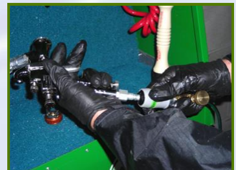
POWERCLEAN™ .... Supply's Compressed Air to the Spray Gun During the Cleaning Process, Protecting the Air Passageways
