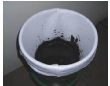
Paint Waste collected by the Filter
